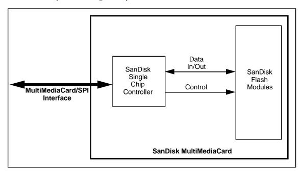
Figure 1-1 MultiMediaCard Block Diagram
