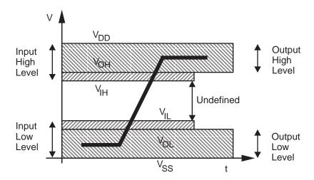
Figure 4-4 Bus Signal Levels
