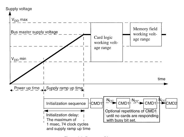
Figure 4-2 Power-up Diagram
