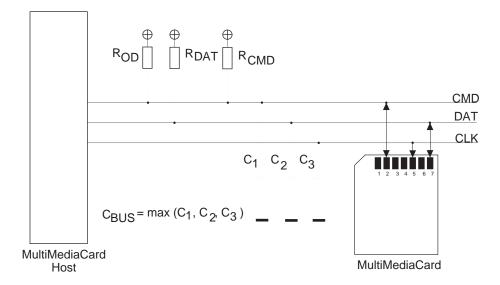
Figure 4-1 Bus Circuitry Diagram
