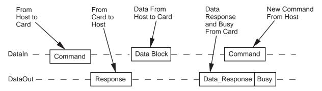
Figure 6-3 Write Operation
