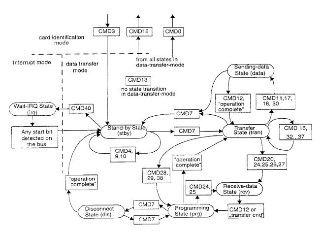
Figure 5-2 MultiMediaCard State Diagram (Data Transfer Mode)
