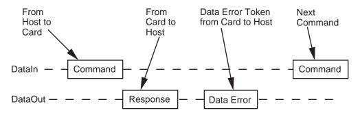
Figure 6-2 Read Operation - Data Error
