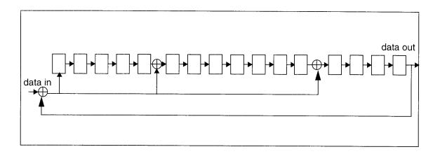
Figure 5-20 CRC16 Generator/Checker
