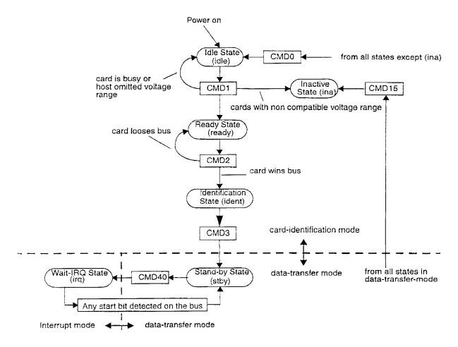
Figure 5-1 MultiMediaCard State Diagram (Card Identification Mode)
