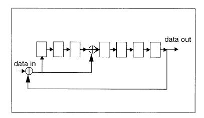
Figure 5-19 CRC7 Generator/Checker
